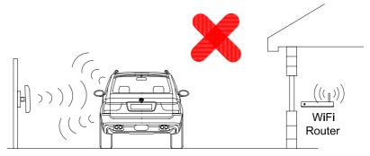
3. For longer range applications, check if the router is, or can be located at the front of the building, preferably near a window or glass, as this will greatly extend range as shown.
