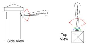
**TIP:** Antenna beam width is approximately 40 degrees. For short range door intercoms, ask your distributor or dealer for an omni-pole type antenna with 360 degree beam angle.
