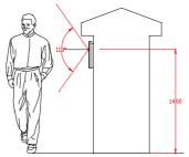
Mount the intercom at the desired height for pedestrian or car users. The camera angle is wide at 110 degrees to cover most scenarios.
