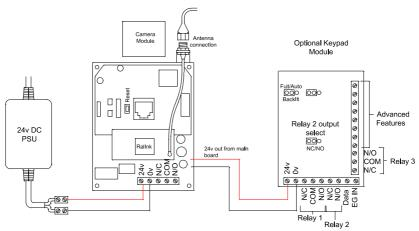
Depending on your requirements, the intercom and keypad have both normally closed and normally open output contacts for connection to existing electric locks or gate automation controllers.
