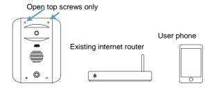
Locate the intercom on a bench or table beside the home router, along with the user phone. Connect the antenna & power supply provided to the intercom, red to +24v dc and black to 0v dc, and power on.
