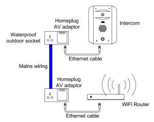
Note: The power to the gate needs to be on the same RCD trip as the power connected to the router for this option to work. Always consult a qualified electrician regarding mains wiring.
